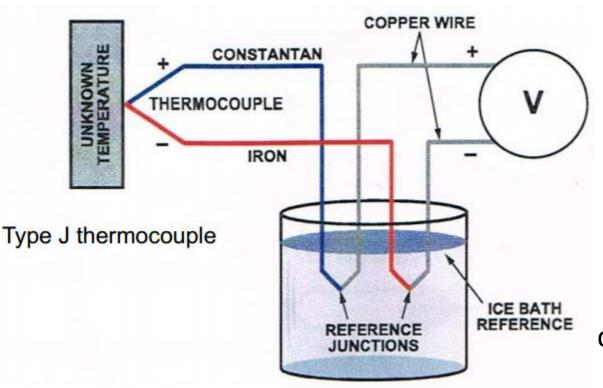
NIST thermocouple reference tables are generated with T<sub>ref</sub> = 0 °C
